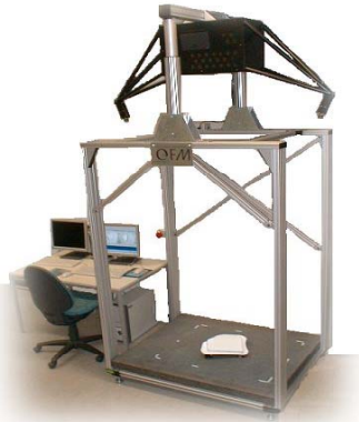
Fig. 3. Two camera fringe projection system.
